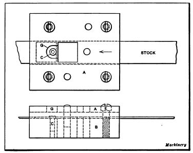
Fig. 31. Improved Form of Fixed Stop-pin
